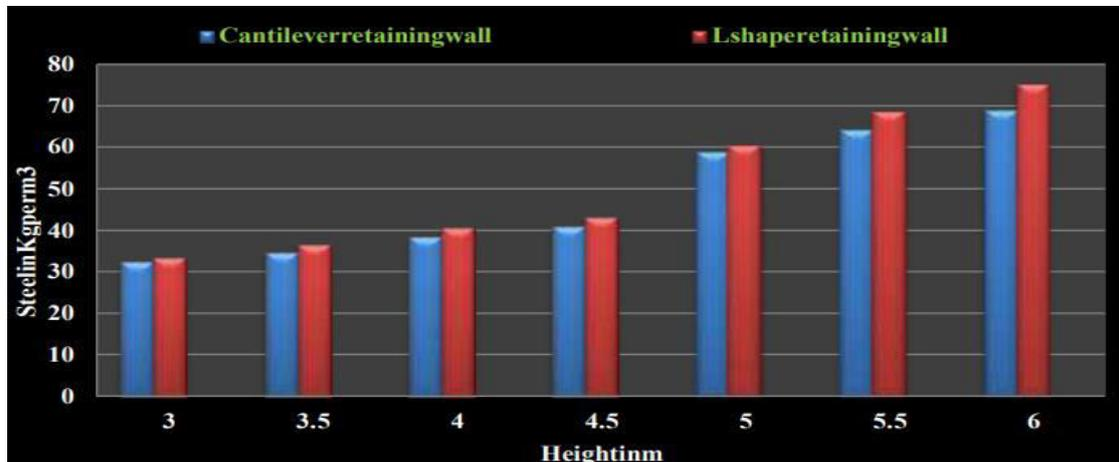
Fig.4: comparison of quantity of steel between Inverted T and L shape wall
