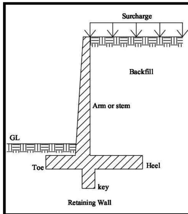
Fig. 1: Cantilever retaining wall
