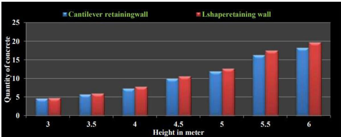
Fig.5: comparison of quantity of concrete between Inverted T and L-shape retaining wall
